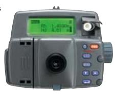
operator can make accurate measurements, and automatic operation eliminates conventional errors arising from misreading or variant results. Extensive field-testing has proven high accuracy with a standard deviation of only 0.6mm for 1km double-run leveling using invar staves, and 1mm using fiberglass staves. The SDL30 has a distance accuracy equivalent to ±1cm at 10m (0.4in. at 33ft.) and ±5cm at 50m (2in at 160ft.).
