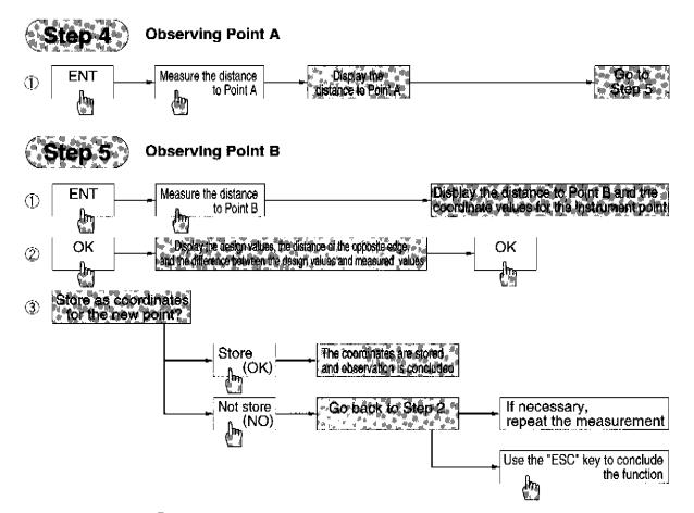
$<sup>^\</sup>star$  If the difference at  ${\hbox{\@red}}$  in Step 5 is excessively large, do the measurement again.
