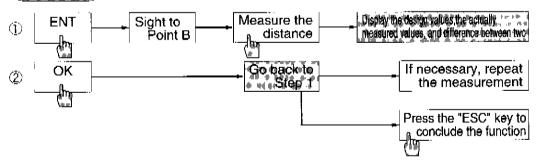
In the remote stake check function, the difference between the design values for a horizontal distance, calculated using inverse calculation from the coordinate values of two known points (Points A and B), and the horizontal distance actually measured between A and B is displayed. The scaling function can also be used with the remote stake check.
