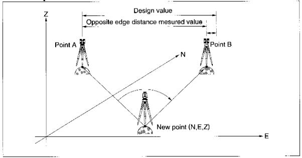
Point ZA: Z coordinate value of the new point obtained by measuring Point ZB: Z coordinate value of the new point obtained by measuring
