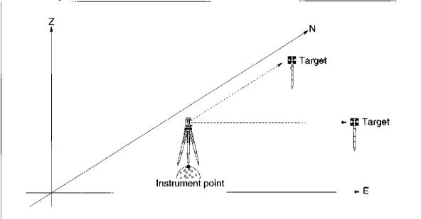
\* When coordinates measurement is done by setting the direction angle to the backsight point, use the Inverse/Azimuth Distance Function to orient the direction angle to the backsight point before measurement.
